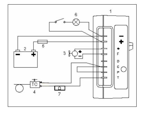
Refrigerator with standard thermostat (12V/24V - 115V/230V)
